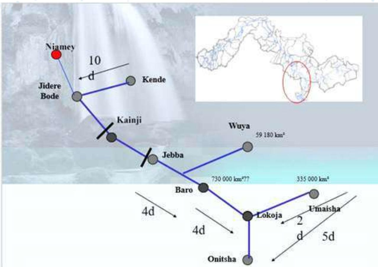
**Figure 2.1: Flow Chart of River Niger from Niamey into Nigeria (showing approximate time of concentration)**
